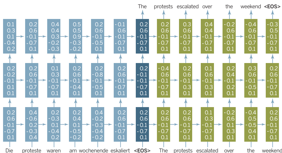
Fig. 2. A deep, recurrent neural MT system (10). Initially trained on parallel sentences that translate each other, the model learns a representation of each word as a real-valued vector and internal parameter matrices so as to optimize translation quality. The trained network can then translate new sentences. Each arrow represents a computation unit of a matrix multiplication followed by a nonlinear transformation; the small vectors shown in the illustration might really be 1000-dimensional. The recurrent network first encodes the meaning of the source sentence (left side, blue). It maintains an internal state representing a partial sentence, which is updated after each new word is read (horizontal arrows). Having the upper network layers [mapped to by additional (upper vertical) computation arrows] makes this a deep recurrent network. Adding depth improves the ability of the model to learn, generalize, and remember. Once the end of the sentence (denoted by <EOS>) is reached (middle, dark blue), the network additionally starts to produce a word of translated output at each step from its internal state (using a multiclass logistic regression-style model). During translation generation (right side, green), the last generated word is fed in as the input at each step. From the stored hidden state and this input, the model calculates the next word of the translation. This process repeats until <EOS> is generated.
